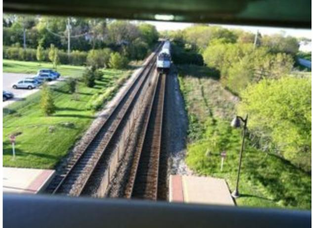
On the way home the engine was in the front of the train. We were pulled to Sturtevant (the train above is heading north) what you see is a cab car at the rear: the prime mover is actually in the front keeping both fume and diesel fuel more or less outside the Chicago station.
